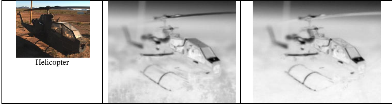
Figure 6. Cross section of static imagery collected. Imagery is normalized within each image to maximize presented contrast with white representing the radiometrically warmest part of the image.
